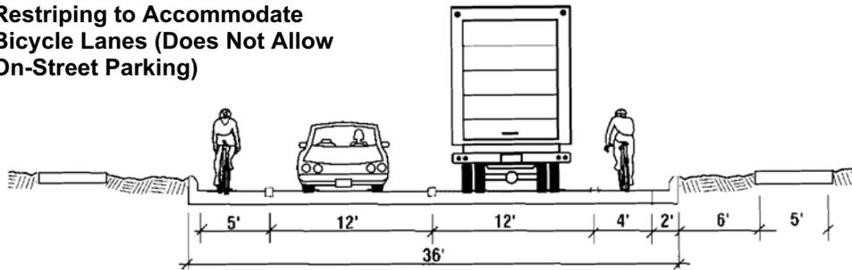
This illustration shows two alternatives for restriping a road on a standard 60' right of way to accommodate bicycle lanes. The left side of the illustration shows a conversion from an 18' travel lane without a 2' gutter pan to a 12' travel lane with a 5' striped bike lane. The right side shows a conversion from a 16' travel lane with a 2' gutter pan to a 12' travel lane, a 4' striped bike lane and a 2' gutter pan.
